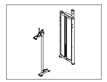
Step 8 Position the Cross Brace to the Main frame.
