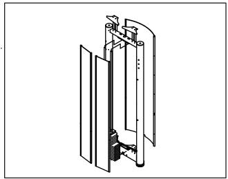
Step 6 Position the Support Frame on the Main Frame and secure it .
