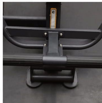
Foot Lever For easy entrance/exit of machine
