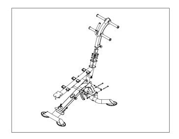
2.Position the round pads and back pad on the frame  $_{\! \circ}$
